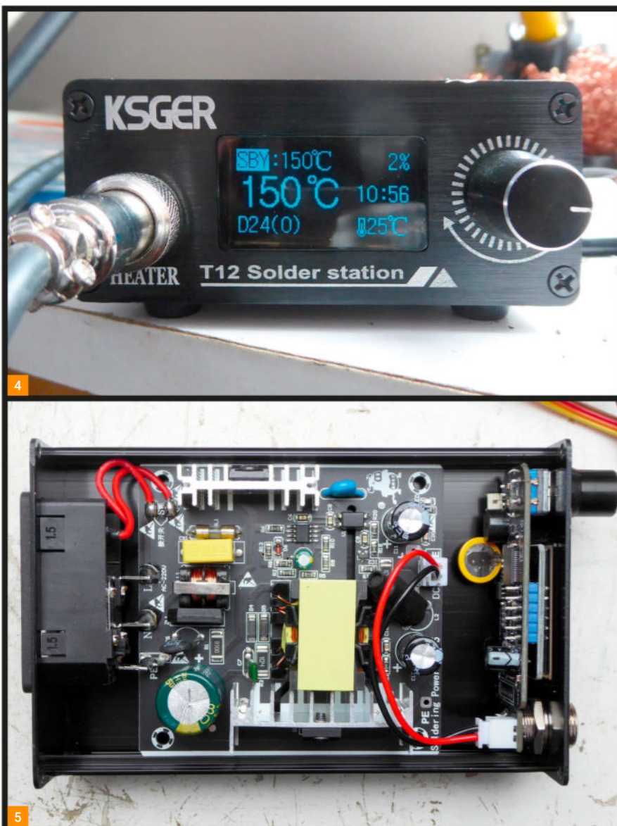
Fig. 1: The KSGER as supplied. Fig. 2: The popular Weller soldering station. Fig. 3: In the hand. Fig. 4: Front Panel showing Standby, Target Temperature of 150°C, Actual Temperature, Percentage power being applied, Fitted tip (D24), CPU Temperature and the time. Fig. 5: Internal view.
