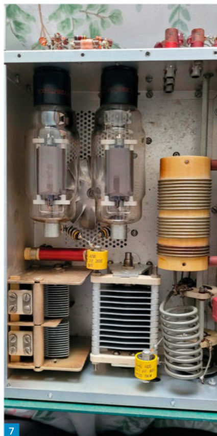
Photo 5: Soft key (left) and soft start (right). Photo 6: Soft start (large) and soft key (small) installed. Photo 7: RF deck after dust removed. Photo 8: Amplifier rear with new connectors. Photo 9: All the old parts removed.
